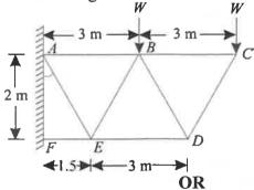
Explain the procedure to find forces in members of truss by using CO5 L2 12M method of joints
