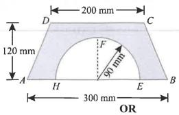
6 Determine the centroid of the area shown in Fig. with respect to the axis CO3 L4 12M shown
